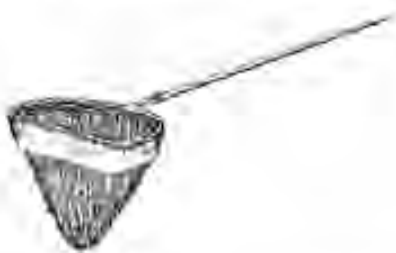
Figure 5-3: D-frame net used for collecting benthic macroinvertebrates.
